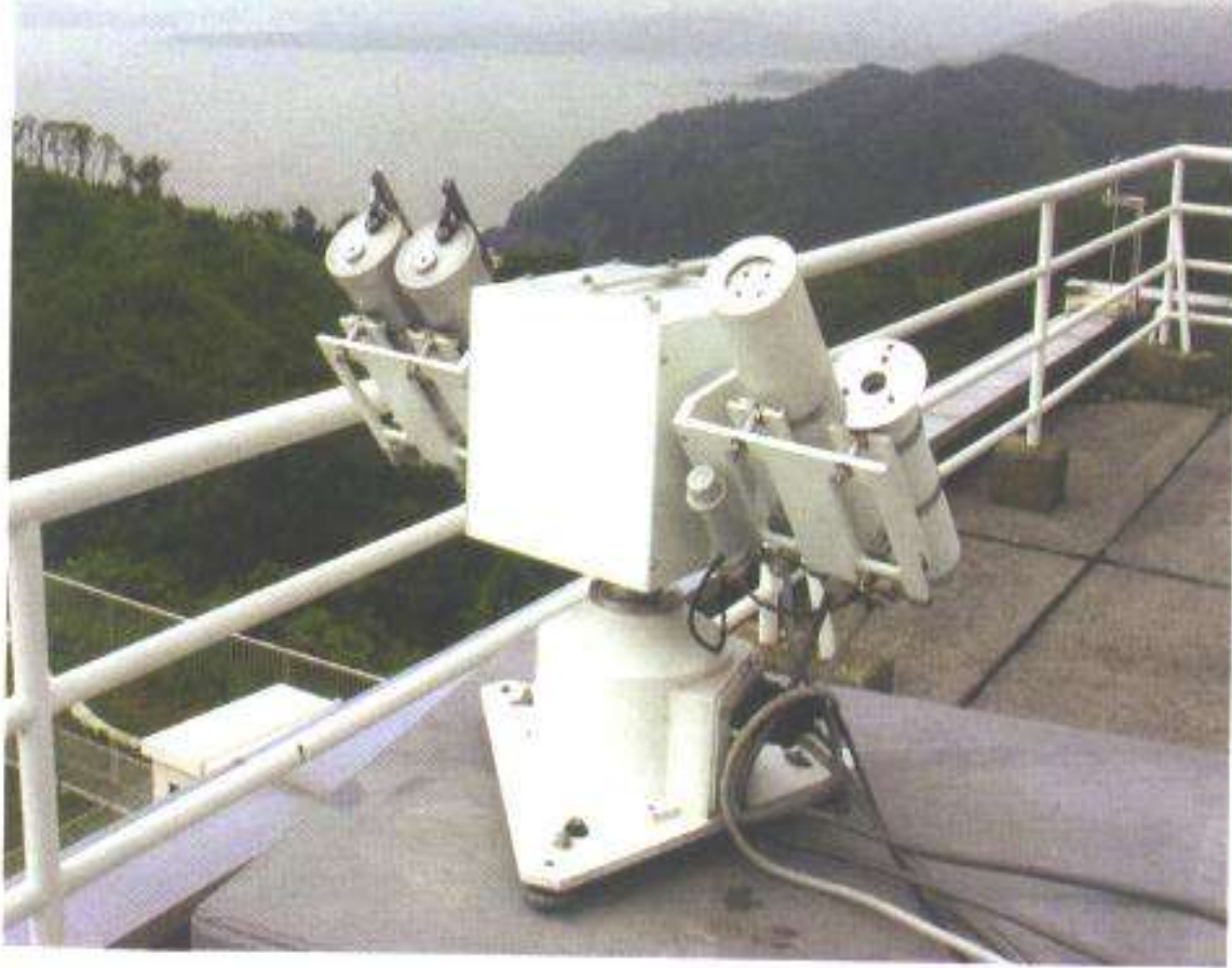
A sun-tracking aerosol photometer at GAW station Ryori, Japan, measures total atmospheric aerosol burden.
