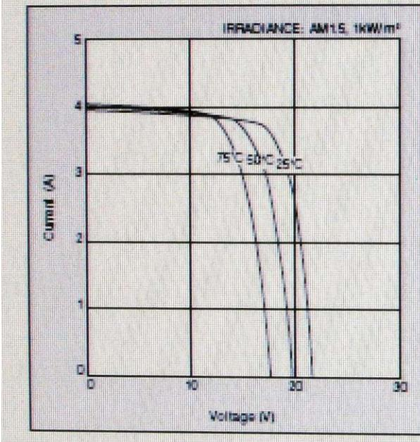
Current-Voltage characteristics of Photovoltaic Module KC65T at various irradiance levels
